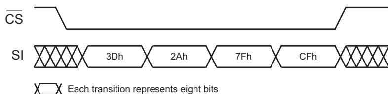
Figure 7-4. Erase Sector Protection Register
